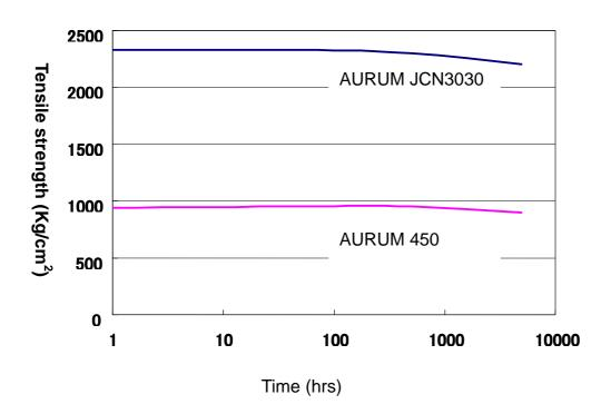
Fig. 1 Changes with Time in Tensile Strength at 230°C
