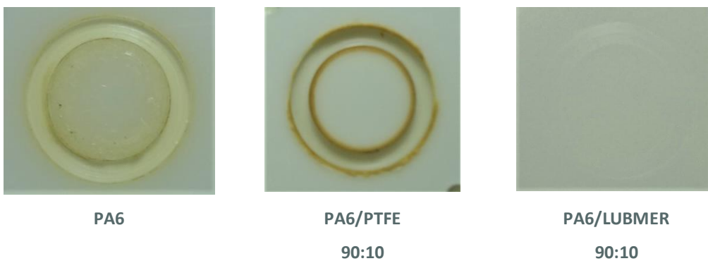
Figure 5: Images showing abrasion loss form test pieces made from pure PA6, PA6 modified with 10% PTFE and PA6 modified with 10% LUBMER™ LY1040
